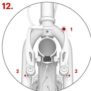
Check that the brake pads move away from the rim sufficiently (1-2 mm) when the brake lever is released. The distance of the brake pads can be adjusted by tightening or loosening the brake cable anchor bolt (1). If the brake pads come into contact with the rim while the wheel spins, adjust the spacing of the brake arms symmetrically with the tensioning bolts (2).
