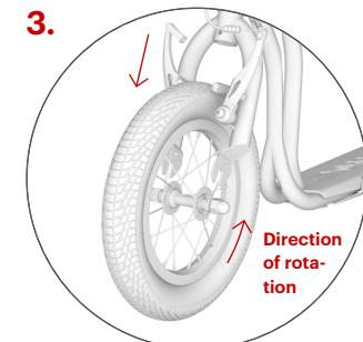
Insert the wheel into the front fork so it is exactly in the middle. **Caution:** When inserting the wheel, ensure that the arrow on the tyre sidewall points in the direction of rotation when the scooter is rolling forwards.
