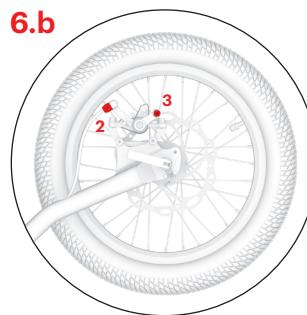
The distance between the pads and the disc should be minimal. You can adjust it with the adjusting roller (2) which regulates the tension of the brake cable. If this is not enough, tighten or even loosen the brake cable at the anchor screw (3).
