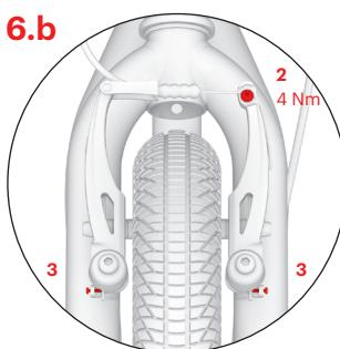
Check that the pads make enough space (1–2 mm) after releasing the brake levers. The distance can be adjusted by tightening or loosening the brake cable at the anchor screw (2).
