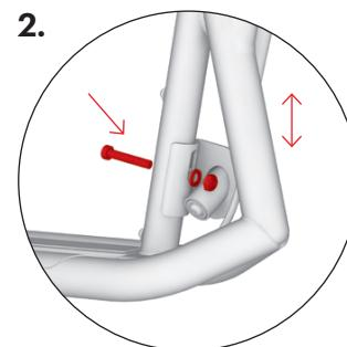
Install the stand attaching it to the frame in front using the prepared hole, see picture. Before tightening the screw, make sure it is placed in the centre of the socket. The oval opening in the socket enables adjusting the height of the stand, so as to provide the model with the greatest possible stability.
