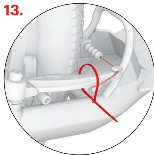
Fasten the end of the brake cable in the lock and secure with the cable tie, then trim the tie (applies to both front and rear brake).
