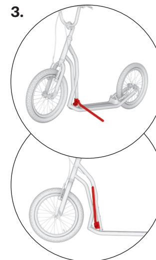
In the riding position, the stand should be aligned with the edge of the scooter frame.
