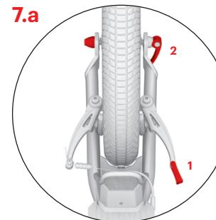
Insert the wheel into the front fork so it is exactly in the middle. **Caution:** When inserting the wheel, ensure that the tyre pattern points in the direction of rotation when the scooter is rolling forwards (on some tyres see direction arrow on the side).
