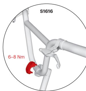
Tighten the adjustment nut of the quick release mechanism to the correct position. When it is in the correct position you will feel a noticeable resistance just before you close the mechanism completely. Close the quick release lever in a position so it does not touch the fork and simultaneously it cannot be opened accidentally while riding.
