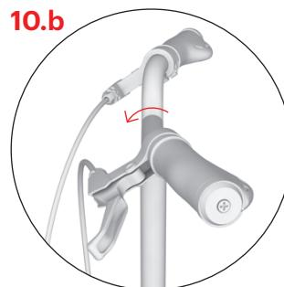
For the best results, stand on the footrest, grab the handlebars and stretch your fingers so they extend in a straight line from your hands. Set the brake levers in this position and tighten the two mounting screws, see 10.a.
